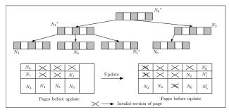
Fig. 2: Update in a  $\mu$ -tree. Updated nodes and new nodes are marked with \* and ' resp. The pages are shown before and after the update.
